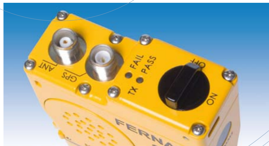
2100 self test and activation LED's.
