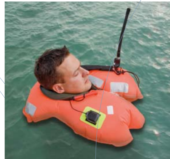
Automatic antenna and GPS patch mounted on life jacket.
